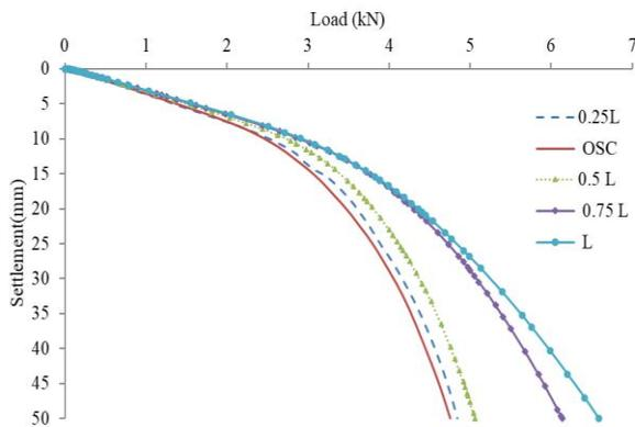
Fig. 6a. Load-settlement characteristics showing the influence of encasement length
