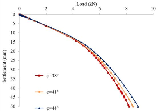
Fig. 5. Load-settlement characteristics showing the effect of varying the friction angle of the column material in GESC
