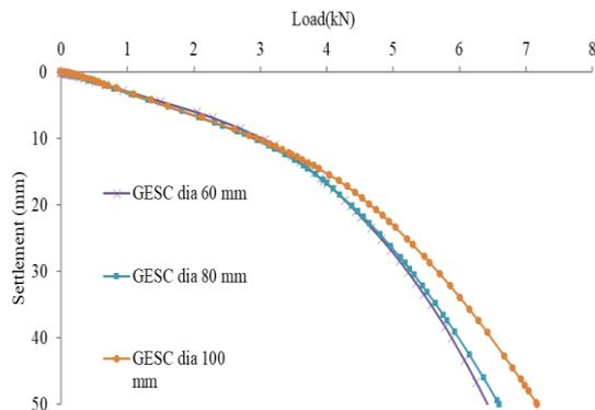
Fig. 4. Load-settlement characteristics of columns of different diameter
