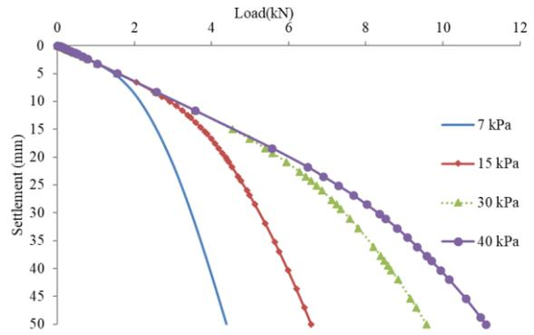
Fig. 8. Load-settlement characteristics of GESC showing the influence of shear strength of clay
