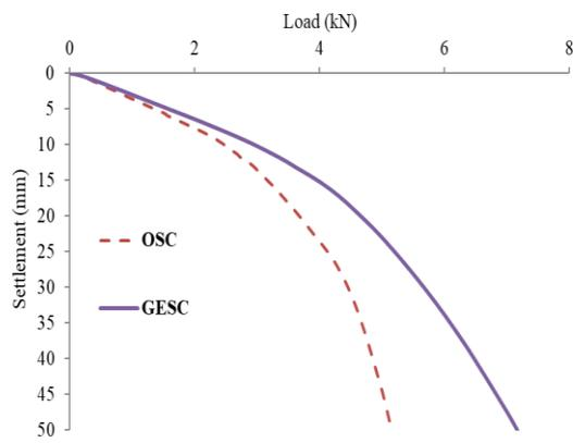
Fig. 3. Comparison of load-settlement characteristics of OSC and GESC
