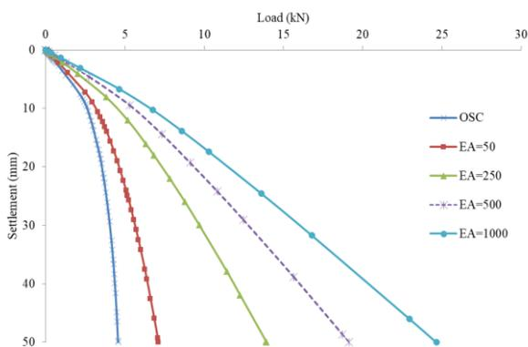
Fig. 7. Load-settlement characteristics showing the influence of stiffness of the geosynthetic encasement
