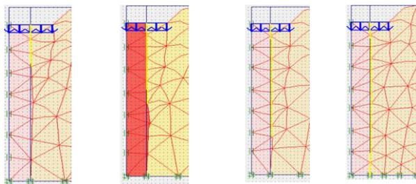
Fig. 6b. Lateral bulging of GESC with different encasing lengths (0.25L, 0.5L, 0.75L, L)
