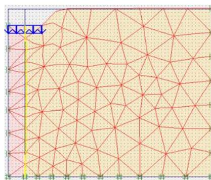
Fig. 1. Deformed mesh, showing the vertical settlement and lateral bulging
