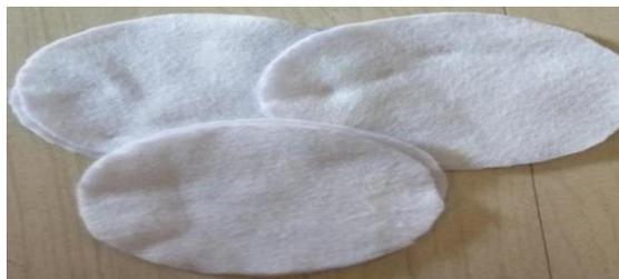
Fig. 2. Non-woven geotextile
