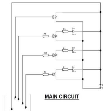
Fig. 1. Circuit of water level indicator
