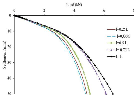
Fig. 4. Load-settlement behavior showing the influence of encasement length ( $L$ - length of the column,  $l$ = encasement length)
