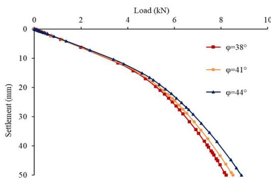
Fig. 2. Load-settlement behaviour of GESC showing the influence of angle of internal friction( $\phi$ ) of the column material
