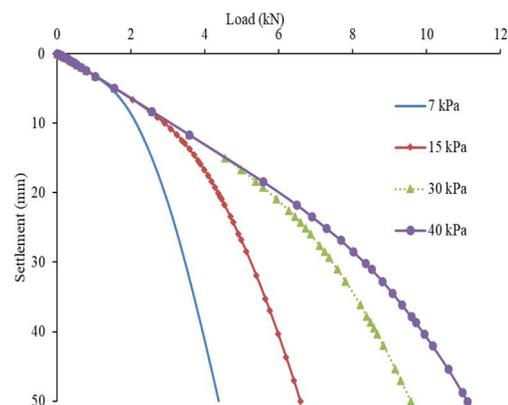
Fig. 5. Load-settlement behavior of GESC showing the influence of shear strength of clay
