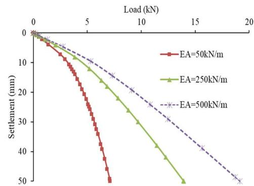
Fig. 3. Load-settlement behaviour of GESC showing the influence of stiffness( $E_A$ ) of the geotextile encasement
