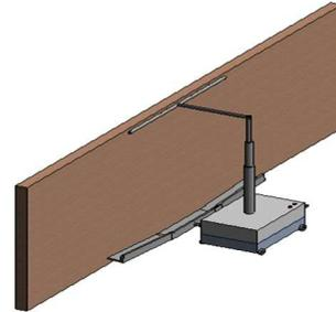
Fig 2: Three-dimensional view of automated curing machine
