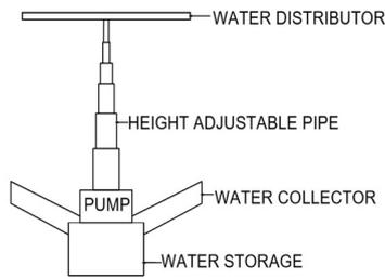
Fig 1: Components of automated curing machine
