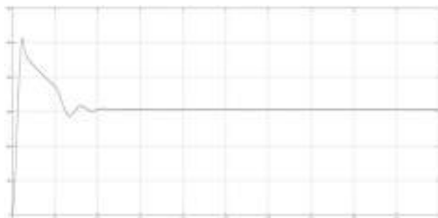
Fig.8. Output voltage of zeta converter
