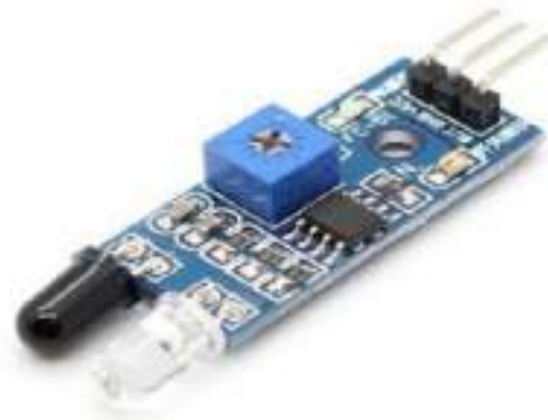
Fig.3. IR Proximity sensor
