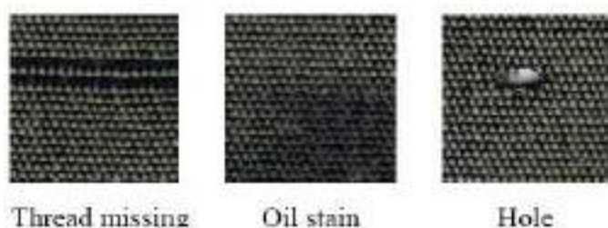
Fig. 1. Examples of defects a) Missing thread b) Oil stain c) Hole
