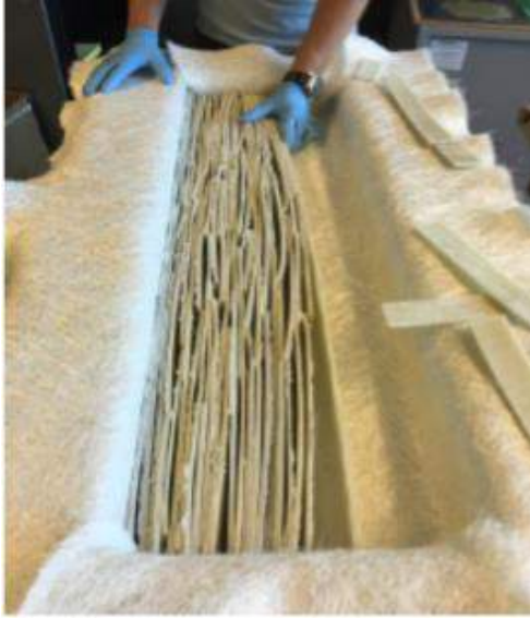
Fig 3.3: Arrangement of fibre panels in the mould
