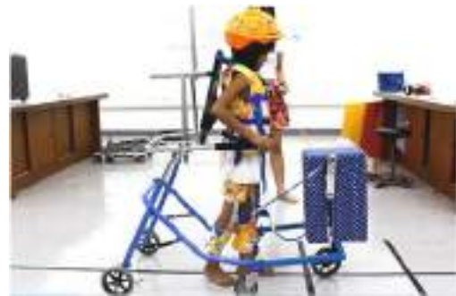
Fig. 2. The prototype of pediatric gait trainer.
