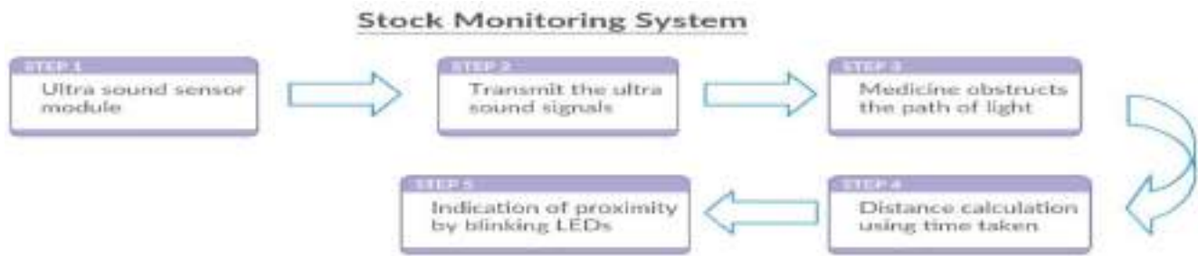
Fig. 4: Block Diagram of Storage Tracking System
