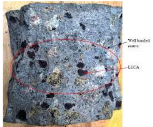
Fig. 6. Failure surface of M3 mix showing well bonded matrix
