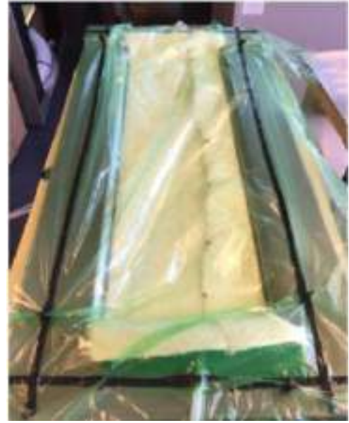
Fig 3.4: Vacuum bagging process
