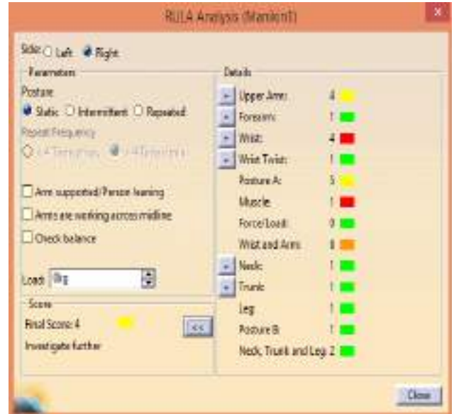
Fig. 7. RULA analysis on 20° Seat Inclination on wheelchair at 0° crank angle of the right side of human
