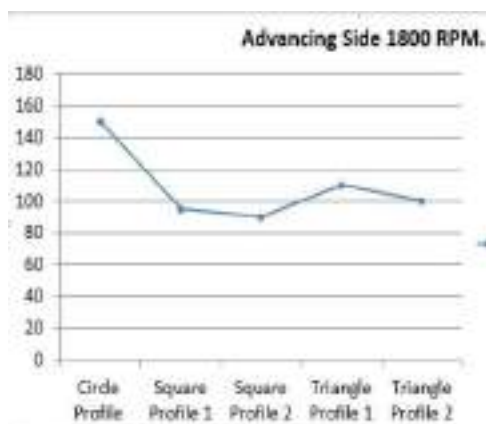
Fig 3.5 Temperature variation in different tool geometry for 1800 rpm in advancing side of stir
