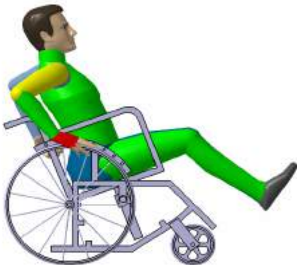
Fig. 6. RULA score on the right side of human body parts of 20° Seat Inclination on wheelchair at 0° crank angle
