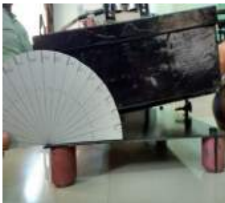
Fig. 12 Measurement of Longitudinal Tilt ( \beta )
