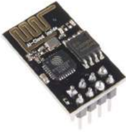
Fig. 3. ESP-8266 Wi-Fi System.
