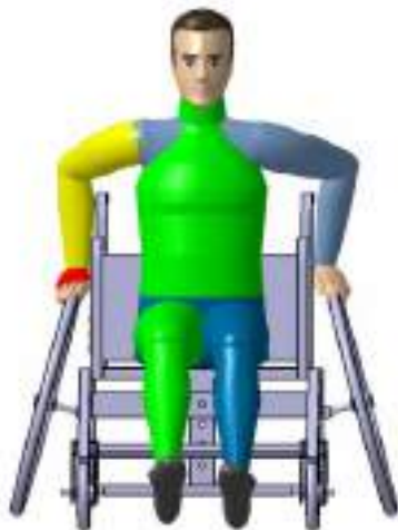
Fig. 8. RULA score on the right side of human body parts of 15° Camber angle of main wheel on wheelchair at 0° crank angle
