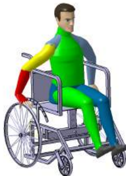
Fig. 4. RULA score on the right side of human body parts on wheelchair seat position 250mm from the main wheel centre on 0° crank angle
