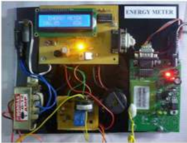
Fig.1. Hardware of Energy Meter
