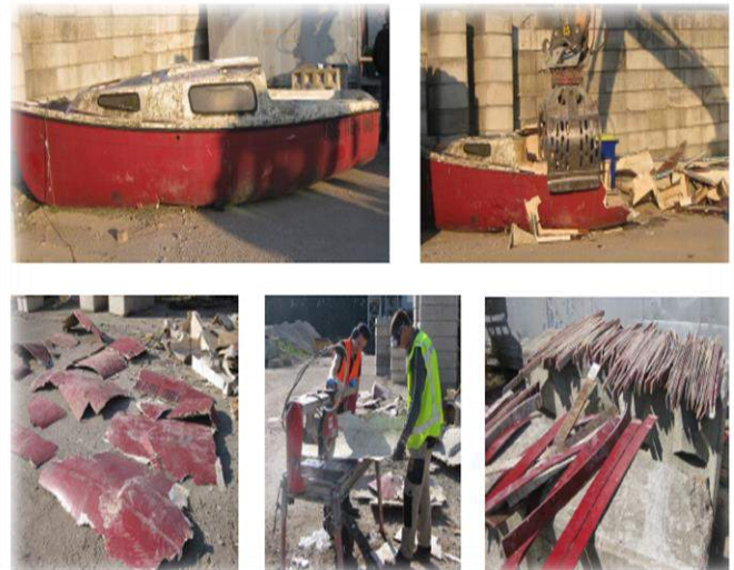
Fig 3.1: Hull of an obsolete boat is processed into large panels
