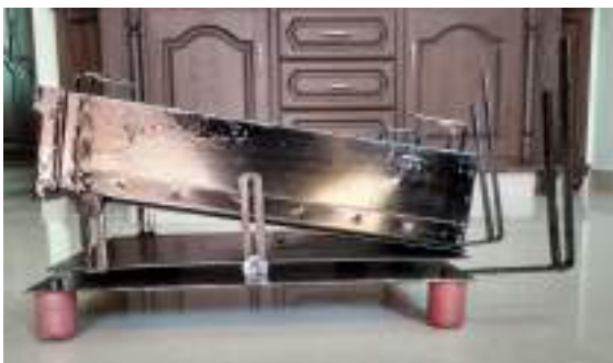
Fig.2 Tank with Tilting Mechanism
