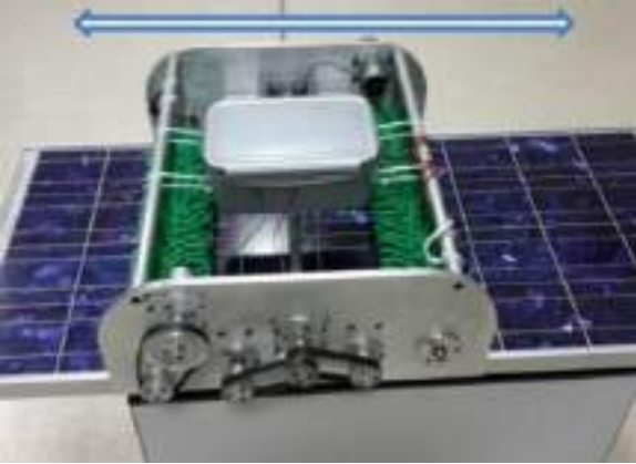
Fig. 6 Direction of cleaning system.
