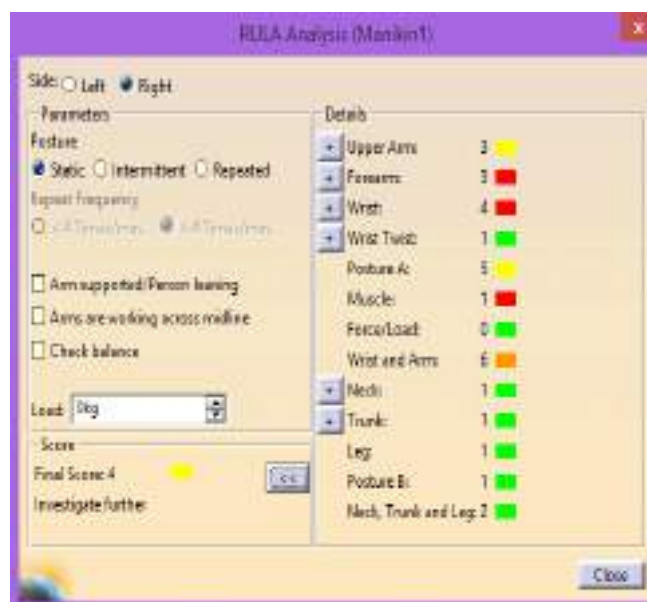
Fig. 5. RULA analysis on the wheelchair seat position 250mm from the main wheel centre on 0° from crank angle at the right side of human
