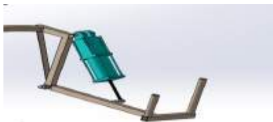
Fig. 1. CAD Model of exoskeleton arm
